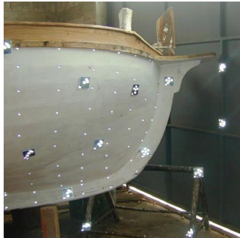
Fig. 1: Preparation of the bow for photogrammetric recording
