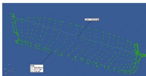
Fig. 3: Result of the photogrammetric measurement, the measuring points define the shape of the boat's hull
