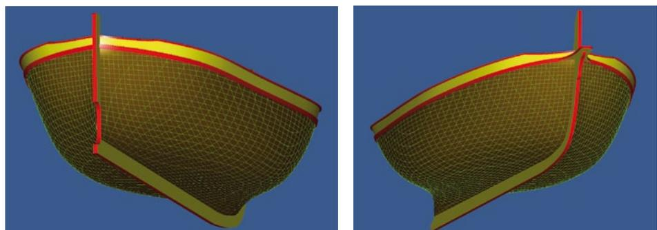
Fig. 5: Characteristic lines (parallel sections) of the boat's hull
