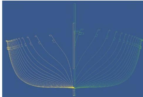
Fig.6: Rib shape, based on the calculated boat model
