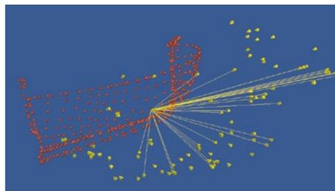
Fig. 2: Reference points (red) and camera positions (yellow) shown in the TRITOP software
