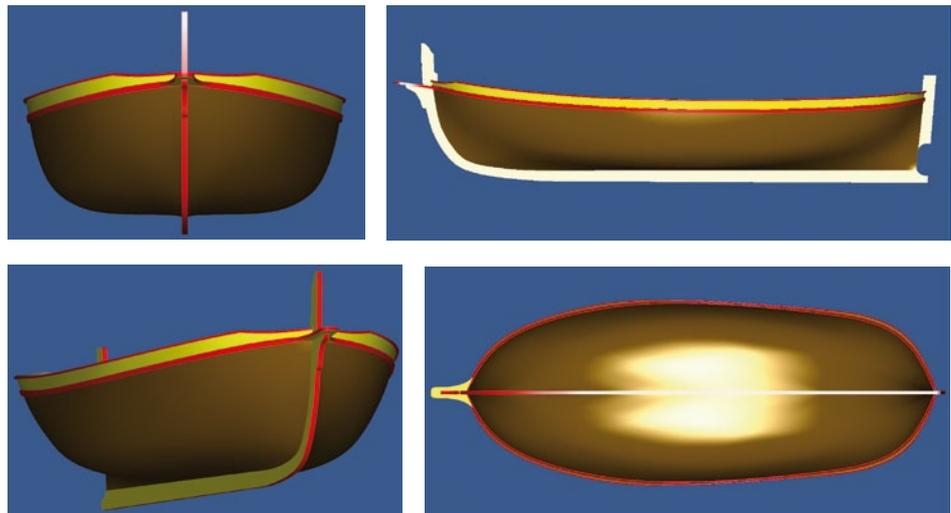
Fig. 4: Calculated CAD model of the boat based on photogrammetric measurement
