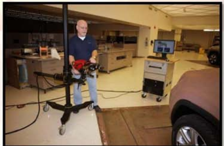
Cliff Kinney, Unit 1 PDO Milling and Digitizing scanning the exterior of a clay model.
