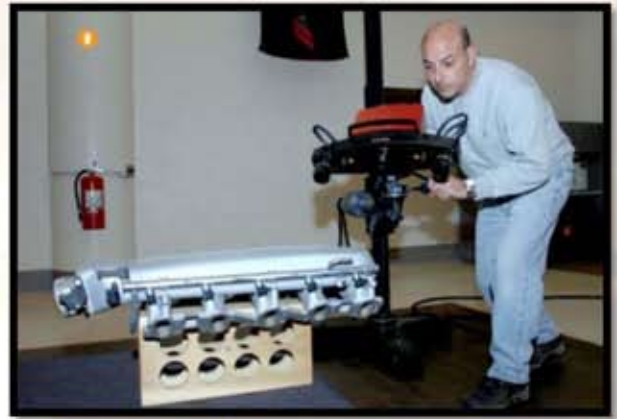
Sam Carnacchi, of VML/PDO Scanning & Imaging scanning a Viper intake manifold.
