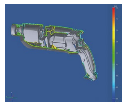
Fig. 4: Deviation of the parting surfaces of a housing part to a plane, warpage of up to 1.2 mm
