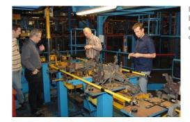
Fig. 1: Welding fixture of a side panel before measuring in the production environment (with Invar scale bars and orientation crosses)
