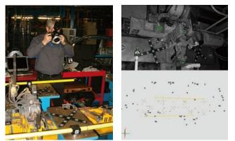
Fig. 4a: Measuring using the TRITOP camera
