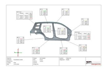
Fig. 6: Measured contact points and their deviation from the nominal position, displayed with CAD data.
