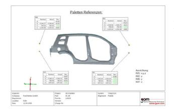
Fig. 5: Measuring the alignment points, visualized together with the CAD data
