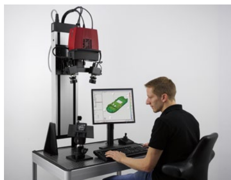
Fig. 1: Digitizing using the ATOS SO system
