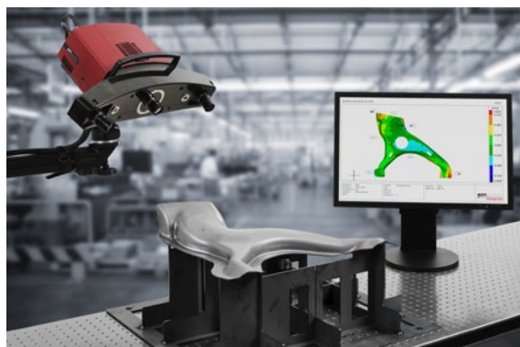
Fig. 2: Mobile optical 3D measurement, component analysis in the production environment
