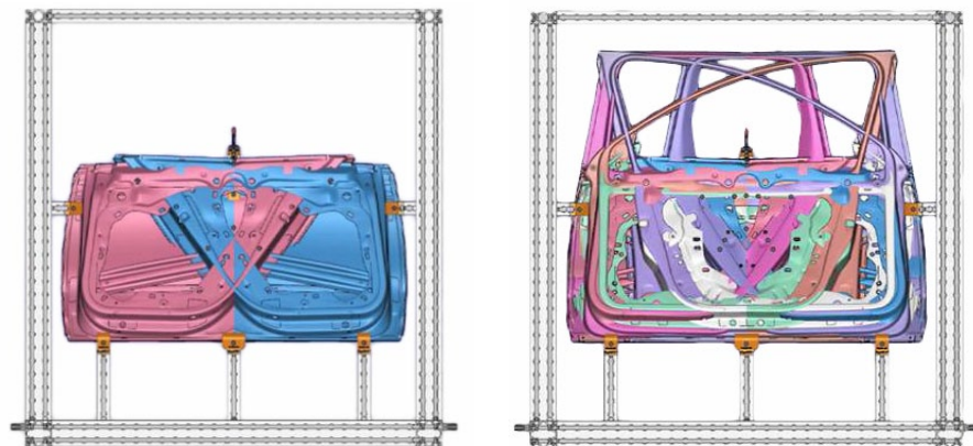
Fig. 7: The optical 3D measuring technique enables the use of an adaptive holder concept that saves on space and costs
