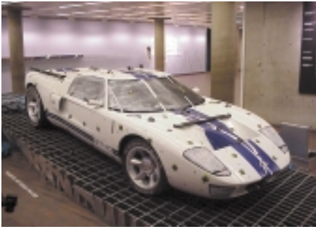
Figure 3 Ford GT40 concept car set up for photogrammetry.
