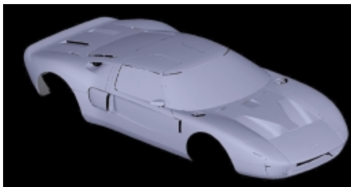
Figure 2b Shaded polygonal mesh from the Ford GT40 concept car scan data.
