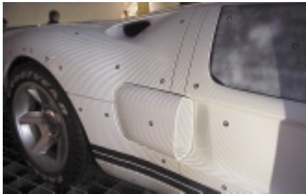
Figure 4a The scanning process of the Ford GT40 concept car.
